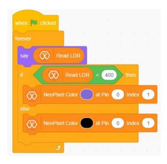
O Adjust the program for different colors in different LDR reading ranges
