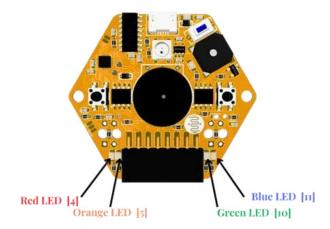
O In Magicbit tiny has four in-built LEDs that can be programmed. These four LEDs have four different colors.
