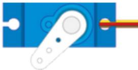
A motor to control the angle of rotation
